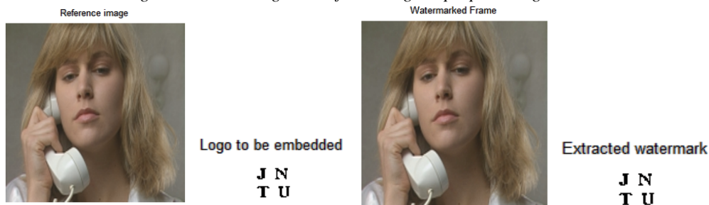
Fig.4:Reference frame, logo image, watermarked frame and extracted watermark
